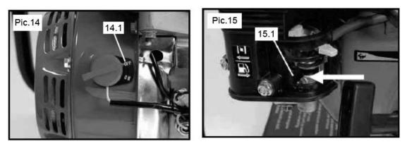
When the engine has stopped and before storage, turns the fuel lever to the OFF position as shown in **Pic.15** (15.1).
