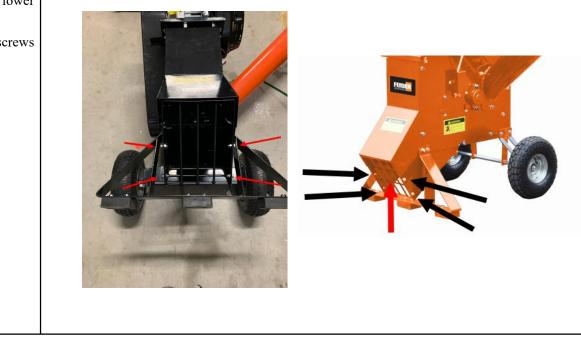
3. Place the handle on the hopper and line up all of the holes. Secure it with flat washer (Ø8, 4pcs), spring washer (Ø8, 4pcs) and bolt (M8x20, 4pcs). (See **Pic.3**)
