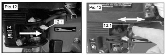
When the engine is running, the speed can be adjusted by moving the throttle control lever (**Pic.13**) (13.1) to the high (indicated by a hare), medium or low position (indicated by a tortoise).
