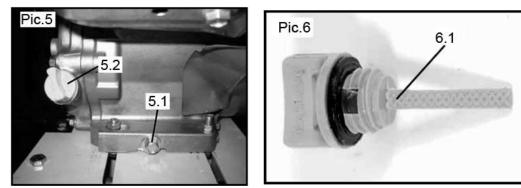
Add engine oil up to the upper level of the dipstick (**Pic.6**) (6.1).
