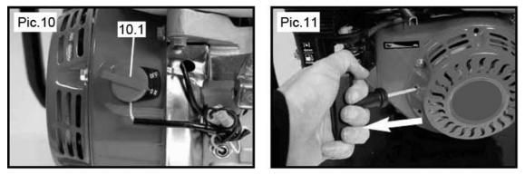
Hold down the engine firmly with one hand on the frame. With the other hand grip the recoil starter cord handle and pull slowly until resistance is felt indicating that the recoil starter is engaged. When resistance is felt pull the cord sharply (**Pic.11**). Continue this procedure until the engine starts.
